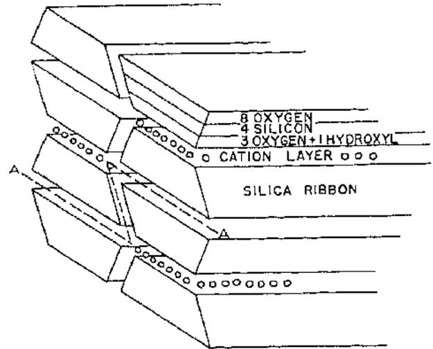
**FIG. 2.** Schematic representation of the chemical structure of amphiboles showing the cation layer which is locked within the I-beam structure (reproduced from Speil and Leineweber (1969), Figure 9, p. 174).
