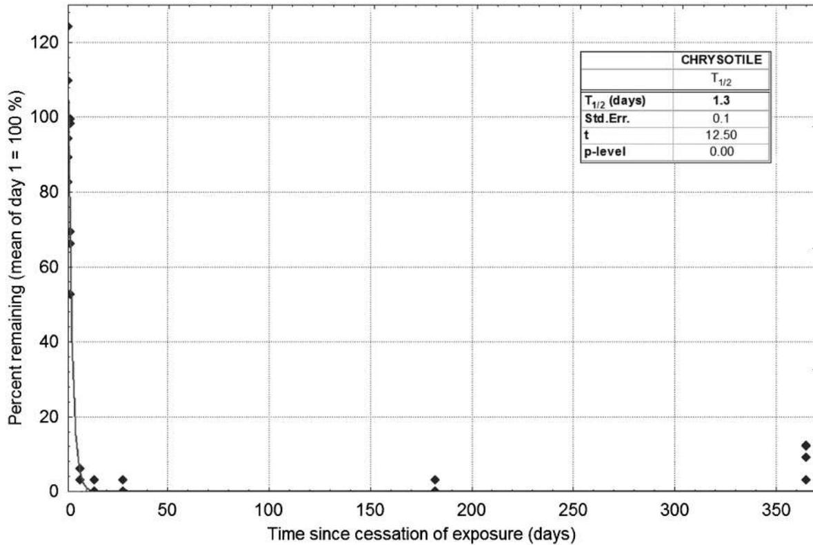
FIG. 5. Biopersistence of chrysotile fibers  $L > 20 \mu\text{m}$ .
