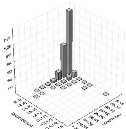
**FIG. 3.** Chrysotile fibers in the exposure atmosphere, bivariate (length and diameter) histogram of WHO fibers.
