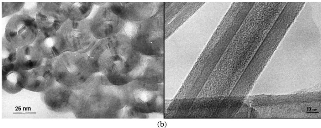
**FIG. 1.** (a) Illustration of the layered structure of chrysotile. From Speil & Leineweber (1969). (b) Transmission electron micrographs of chrysotile showing the coiled sheet like form of the fibers (Cruxên Barros de Oliveira, 1989).
