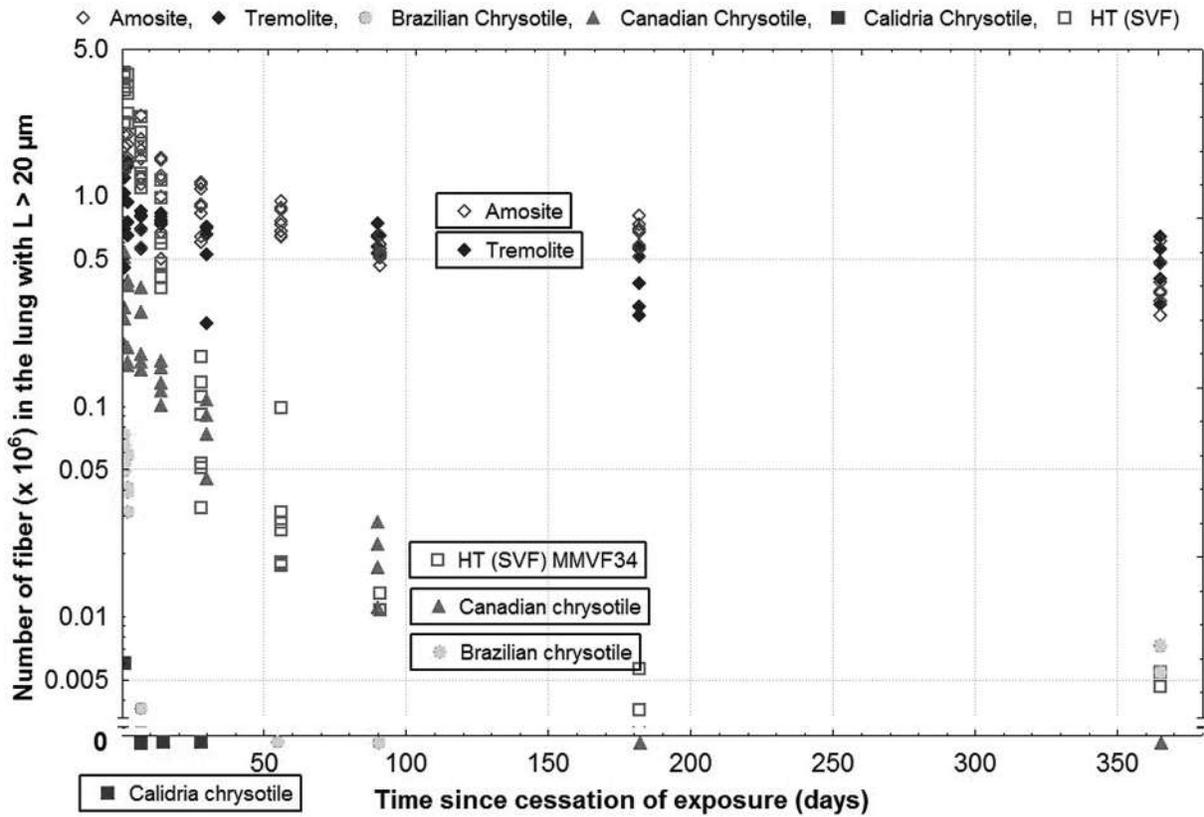
FIG. 12. Biopersistence of chrysotile, amphibole, and SVF: clearance of fibers with length greater than 20 μm.
