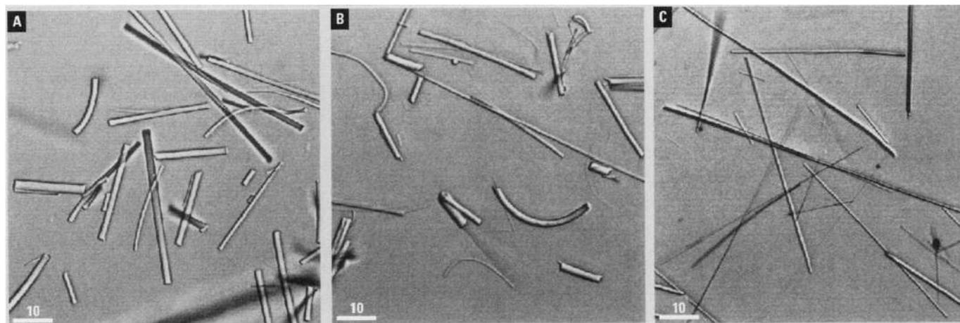
**Figure 1.** Three types of fibers before aerosolization imaged by confocal laser scanning microscopy operated in reflected light mode. Individual fibers of all types appear to be of constant diameter. (A) Man-made vitreous fiber (MMVF)10a: fibers appear somewhat narrower and more curved than MMVF33. (B) MMVF33: note aggregates of individually straight fibers. (C) Long amosite: straight fibers, apparently little aggregated. Bars represent 10  $\mu\text{m}$ .
