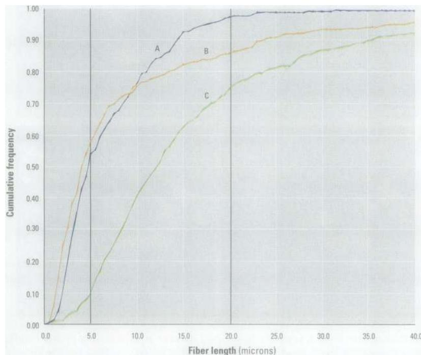
**Figure 8.** Fiber length cumulative frequency distributions of three types of fibers retained in lung after 13-week exposure as determined *in situ* in three dimensions by confocal laser scanning microscopy. Curve A, man-made vitreous fiber (MMVF)10a; curve B, MMVF33; curve C, long amosite (high dose).
